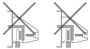
• Strip the cable end long enough (30 mm  $\pm$  5 mm) to be fully clamped. Otherwise, its outer jacket prevents the cable conductor from being tightly secured, causing poor contact.
