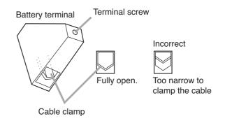
• Insert the battery cable into the correct position in the battery terminal referring to the terminal's cross sectional diagrams below.
