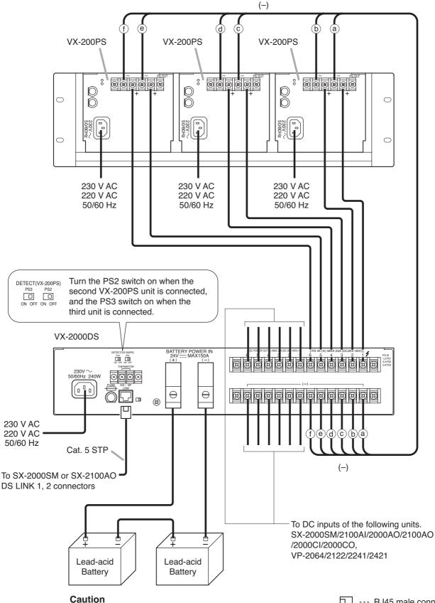
The charging current from VX-2000DS is 5 A maximum. Applicable Batteries: Panasonic LC-X1265PG/APG
