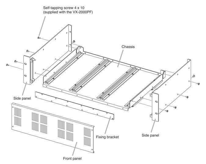
Note: Mount the front panel and fixing bracket after installing the VX-200PS units on the chassis.
